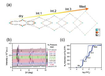
Fig. 3 (a) Scheme of the continuous breathing behavior of the Co(BDP) during N2 adsorption. (b) In situ X-ray powder diffraction patterns of Co(BDP) measured under different gas pressure at 100 K. (c) N<sub>2</sub> adsorption isotherm measured at 77 K, indicating the five pressure-dependent phases. Filled and empty symbols represent adsorption and desorption, respectively. Modified and reprinted with permission from ref. 58.
