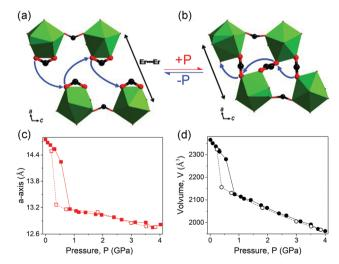
Fig. 19 Partial crystal structure changes of the [tmenH<sub>2</sub>][Er(HCOO)<sub>4</sub>]<sub>2</sub> before (a) and after (b) compression. Lattice parameter changes of a (c) and volume (d). The data collected with increasing and decreasing pressure are plotted with filled and empty spheres, respectively. Reprinted with permission from ref. 124
