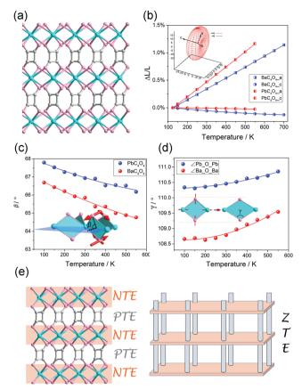
Fig. 9 (a) Crystal structure of pillar-layered  $MC_4O_4$  (M = Ba, Pb). (b) Lattice parameter changes of the  $MC_4O_4$  (M = Ba, Pb) obtained from Le bail fitting. Illustration of the out-plane rotation (c) and geometric deformation (d) of rhombic Pb<sub>2</sub>O<sub>2</sub> (or Ba<sub>2</sub>O<sub>2</sub>) plane. (e) Scheme of the mechanism of 1D ZTE which concerns of the NTE in the inorganic layers and PTE of the organic pillar. Reprinted with permission from ref. 84.
