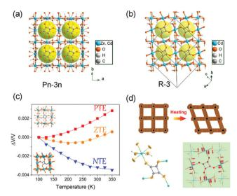
Fig. 11 Crystal structure of the cubic phase (a) and trigonal phase (b) of  $MC_4O_4 \cdot 2H_2O$  (M = Zn, Cd). (c) Temperature-dependent relative volume changes of the three compounds. (d) Scheme of the wine-rack distortion of the framework in the trigonal phase Cd\_sq\_R and illustration of the transverse vibration of the squarate ligand. Reprinted with permission from ref 93
