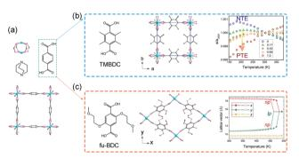
Fig. 8 (a) Crystal structure of the  $Zn_2(BDC)$  (dabco) viewing along the c axis and its building units. (b) Illustration of the structure after TMBDC decoration and the lattice parameter changes as a function of temperature and composition. (c) Illustration of the structure after fu-BDC decoration and the temperature-dependent lattice changes. Partly taken from ref. 70 and 71 with permission.
