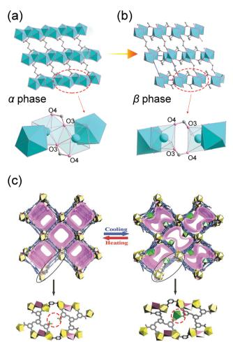
Fig. 13 Illustration of the structural changes of  $[Yb_2(C_4H_4O_4)_3]$  at low (a) and high (b) temperatures. Top: The overview of the framework. Bottom: Local SBU changes. (c) Scheme of the temperature induced structural changes. Top: The overview of the 3D framework. Bottom: The local enlarged view of the structural difference. Partly taken from ref. 99 and 100 with permission
