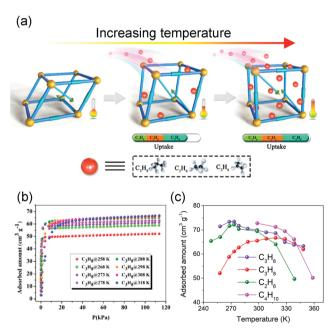
Fig. 5 (a) Scheme of the enhanced gas adsorption in NKU-FlexMOF-1. (b) C<sub>3</sub>H<sub>8</sub> adsorption isotherms from 258 to 318 K. (c) Temperaturedependent uptake amounts for C<sub>2</sub>H<sub>6</sub> (green), C<sub>3</sub>H<sub>6</sub> (purple), C<sub>3</sub>H<sub>8</sub> (red) and C<sub>4</sub>H<sub>10</sub> (pink). Reprinted with permission from ref. 61.
