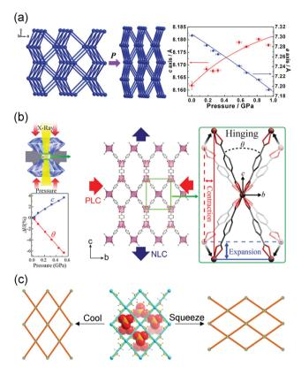
Fig. 16 Scheme of the wine-rack structural changes under hydrostatic pressure that exhibit NLC. (a)  $[NH_4][Zn(HCOO)_3]$ . (b)  $InH(BDC)_2$ . (c) [Ag(ethylenediamine)]NO<sub>3</sub>. Partly taken from ref. 111, 113, and 116 with permission
