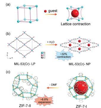
Fig. 2 (a) Scheme of the guest insertion induced lattice contraction. Illustration of the crystal structure changes of MIL-53 (b) and ZIF-7 (c) during the guest insertion and desolvation. Partly taken from ref. 15 and 55 with permission.
