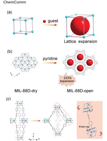
Fig. 1 (a) Scheme of the guest insertion induced lattice expansion. (b) Crystal structure of the MIL-88D before and after pyridine loading. (c) The cage structure in MIL-88D before (left) and after (middle) guest loading. Right: Illustration of the framework displacements during swelling, which occur around the knee cap O–O axis (blue lines and green arrows). This allows the rotation around this axis of the whole trimeric units (red arrows). Partly taken from ref. 19 with permission.
