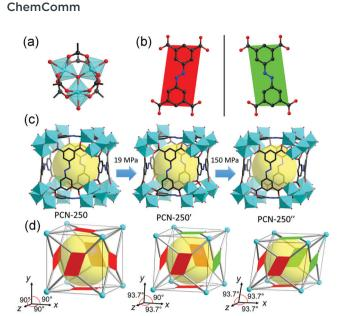
Fig. 20 (a) Structure of the  $Fe_3$ -oxo cluster. (b) ABTC ligand with two different kinds of configurations. (c) Crystal structure of PCN-250 at different pressures. (d) Scheme of the pressure induced structural transformation including the inclination of unit cell and flipping of ligands. Reprinted with permission from ref. 126.
