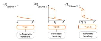
Fig. 15 Illustration of the possible volume change of a material under hydrostatic pressure. (a) Type 1: continuous volume decrease without framework transition. (b) Type II, an irreversible abrupt volume decrease at a certain pressure. (c) Type III, reversible breathing. Reprinted with permission from ref. 103.
