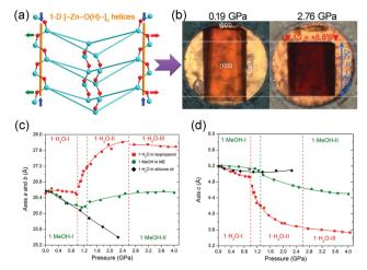
Fig. 17 (a) A perspective view of the quadrangular rings connected by the  $[-Zn-O(H)-]_n$  helices to form a column along the c axis. (b) Photograph of a single crystal of  $[Zn(L)_2(OH)_2]\cdot H_2O$  compressed in isopropanol in the diamond-anvil cell (DAC) chamber. Lattice parameter changes along a axis (c) and c axis (d). Reprinted with permission from ref. 117.
