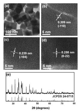
Fig. 3 (a) TEM image of  $Ag_2S$  nanocubes obtained at 72 h and (b-d) their HR-TEM images showing d-spacing of (-110), (-104), and (0-22) crystal facets. (e) XRD pattern of the Ag<sub>2</sub>S nanocubes.
