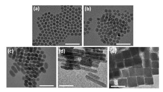
Fig. 1 TEM images of  $Ag_2S$  NPs obtained at different time points: (a) 2 h, (b) 6 h, (c) 24 h, (d) 30 h, and (e) 72 h (all the scale bars 50 nm).
