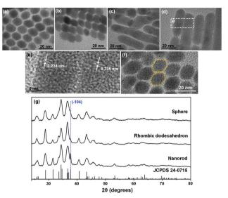
Fig. 2 TEM images of  $Ag_2S$  NPs obtained at 24 h: (a) DHNCs, (b) nanodumbbells, (c) NRs. TEM image of  $Ag_2S$  NPs obtained at 30 h: (d) NRs, HRTEM image of the dotted box as (e), showing d-spacing of (-104) crystal facet. (f) Representative TEM image of  $Ag_2S$  DHNCs facing each other along the (-104) planes, (g) XRD data of different shape of NPs.
