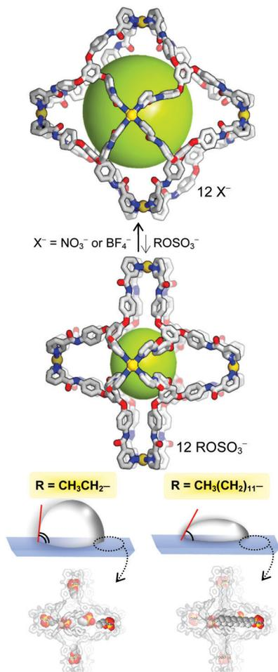
**Scheme 1** Encapsulation of  $\text{ROSO}_3^-$  (R = ethyl-, octyl-, decyl-, dodecyl-, and tetradecyl-) within present spherical coordination cages and different surface tensions depending on included alkyl chains of surfactant.
