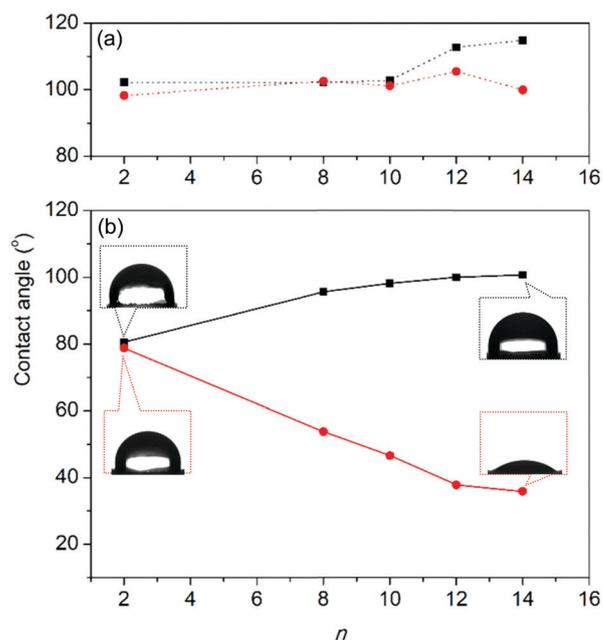
Fig. 3 Surfactant responsive contact angles on fine-ground crystal surface of  $2:12\text{C}_n\text{H}_{2n+1}\text{OSO}_3$  at 0 min (a) and after 10 min (b) (black line: drop of  $\text{H}_2\text{O}$ ; red line: mixture solution of water and ethanol (4:1)).
