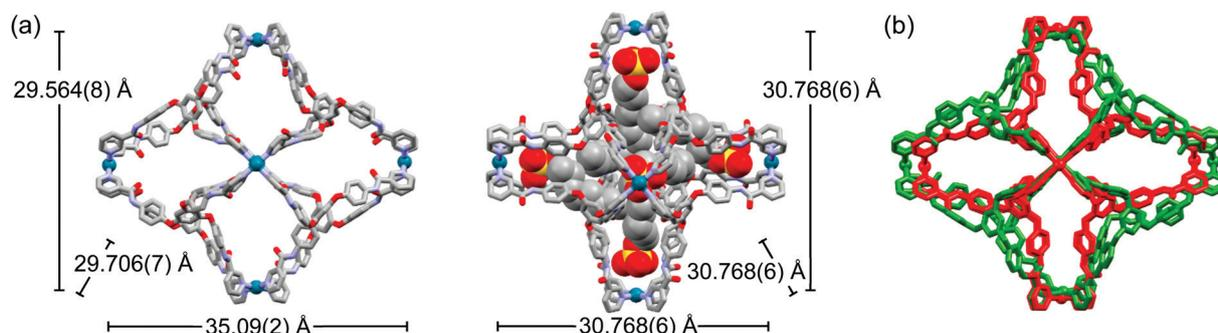
**Fig. 1** Crystal structures and Pd $\cdots$ Pd distances for  $1\cdot 12\text{NO}_3$  (a, left) and  $2\cdot \text{C}_8\text{H}_{15}\text{OSO}_3$  (a, right). Overlay (b) of  $1\cdot 12\text{NO}_3$  (green) and  $2\cdot \text{C}_8\text{H}_{15}\text{OSO}_3$  (red).
