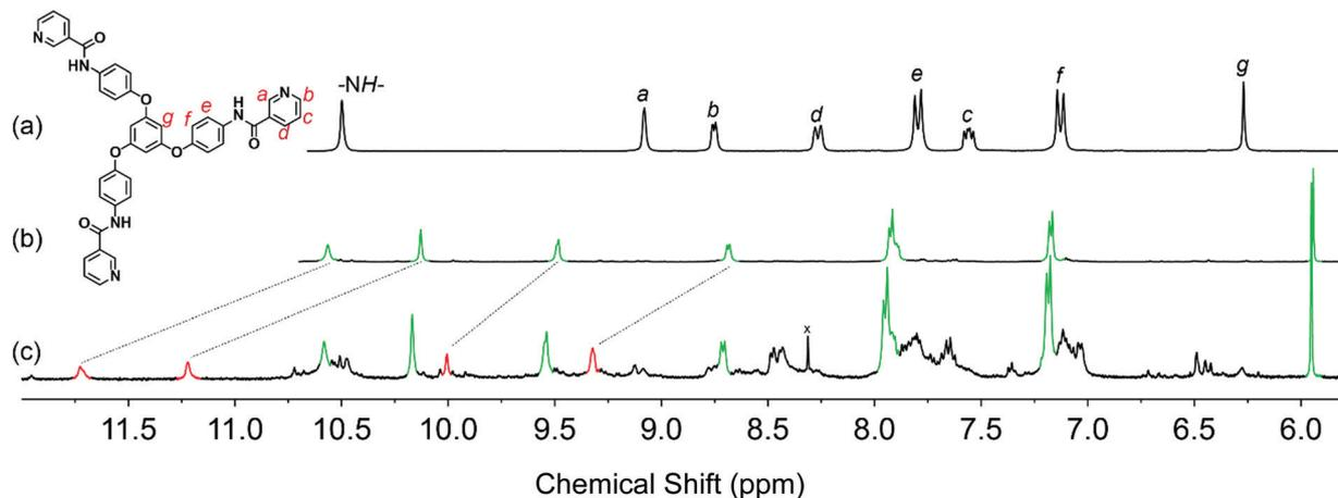
Fig. 2  $^1\text{H}$  NMR spectra for L (a),  $1:12\text{NO}_3$  (b), and after addition of 12 equiv. of  $\text{NaC}_{12}\text{H}_{25}\text{OSO}_3$  into  $1:12\text{NO}_3$  (c) in  $\text{Me}_2\text{SO}-d_6$ . The  $1:12\text{NO}_3$  and  $2:12\text{C}_{12}\text{H}_{25}\text{OSO}_3$  resonances are indicated by the green and red signals, respectively.
