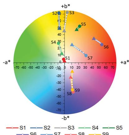
Fig. 4 Color tracks obtained for **S1–S9** when titrating against  $\text{Na}^+$  ( $\text{Na}^+ = 0$  mM denoted by filled circle,  $\text{Na}^+ = 6.66$  mM denoted by filled triangle, with increments of 0.66 mM noted by white filled circles).
