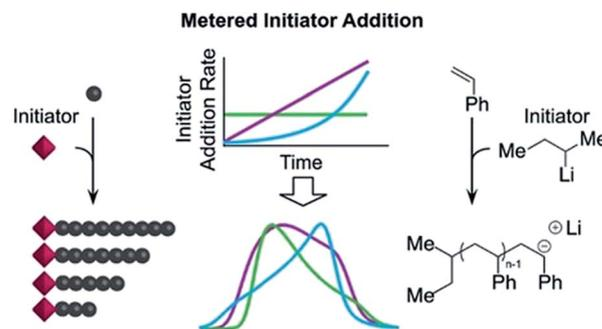
Fig. 3 Tailored shape and dispersity of the molecular weight distribution, produced *via* metered addition of *s*-BuLi to the anionic polymerisation of styrene. This figure is adapted from ref. 56 with permission from ACS publications.
