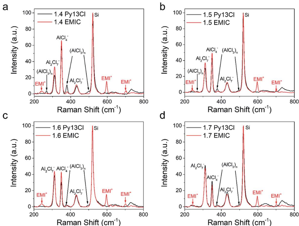
Fig. 3 Raman spectra comparison between Py13Cl–AlCl<sub>3</sub> and EMIC–AlCl<sub>3</sub> ionic liquid. (a) 1.4 Py13Cl and 1.4 EMIC comparison, (b) 1.5 Py13Cl and 1.5 EMIC comparison, (c) 1.6 Py13Cl and 1.6 EMIC comparison, (d) 1.7 Py13Cl and 1.7 EMIC comparison.
