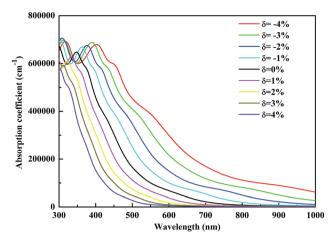
Fig. 7 Calculated optical absorption coefficients of CsGel<sub>3</sub> under different strain conditions.
