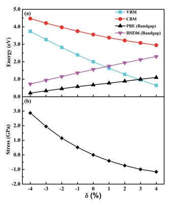
Fig. 4 (a) VBM, CBM, bandgap and (b) stress of CsGel<sub>3</sub> as a function of strain.
