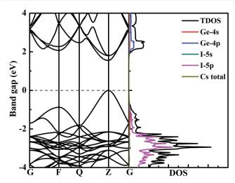
Fig. 3 The band structure and density of states of CsGel<sub>3</sub> calculated at the HSE06 level
