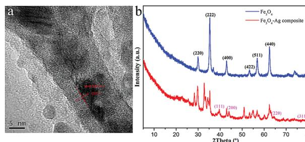
Fig. 4 HRTEM image of Ag nanowires (a) and XRD patterns of the Fe<sub>3</sub>O<sub>4</sub>-Ag nanocomposite (b).
