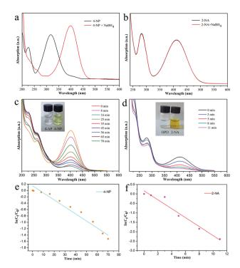
Fig. 7 The spectra of 4-NP and 2-NA with the addition of NaBH<sub>4</sub> (a and b). Curves of the catalytic reduction of 4-NP (c) and 2-NA (d). Plots of  $\ln(C_t/C_0)$  versus time for 4-NP (e) and 2-NA (f). Pictures (insets in (c) and (d)) represent the solutions before/after the catalytic reaction.
