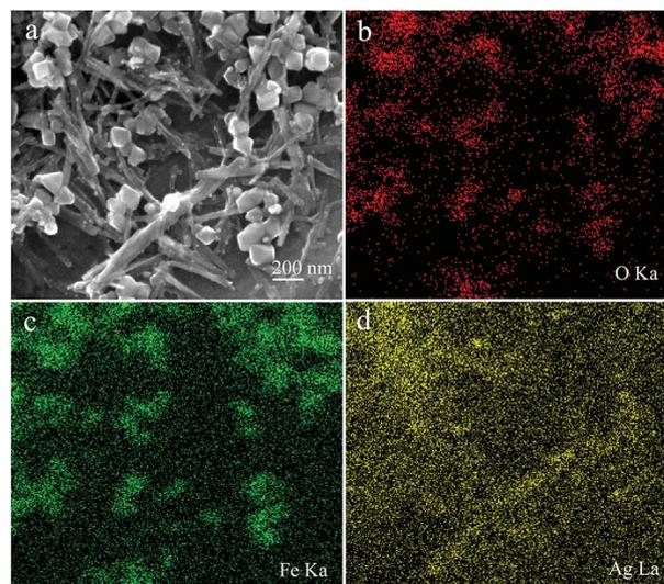
Fig. 3 SEM image (a) and O/Fe/Ag (b, c, and d) elemental mapping of the obtained Fe<sub>3</sub>O<sub>4</sub>-Ag nanocomposite.
