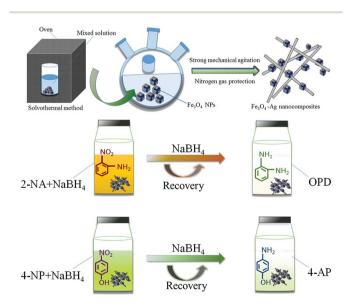
Fig. 1 Schematic illustration of the preparation and catalytic performances of the obtained Fe<sub>3</sub>O<sub>4</sub>-Ag nanocomposite.
