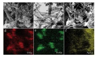
Fig. 9 SEM (a) and TEM (b) images with O/Fe/Ag elemental mapping (d, e, and f) of the  $Fe_3O_4$ -Ag nanocomposite after eight consecutive cycles of catalytic reactions.
