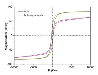
Fig. 5 Magnetization hysteresis loops of as-prepared  $Fe_3O_4$  nanoparticles and  $Fe_3O_4$ -Aq nanocomposite.
