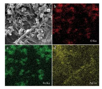
Fig. 3 SEM image (a) and O/Fe/Ag (b, c, and d) elemental mapping of the obtained  $Fe_3O_4$ -Ag nanocomposite.
