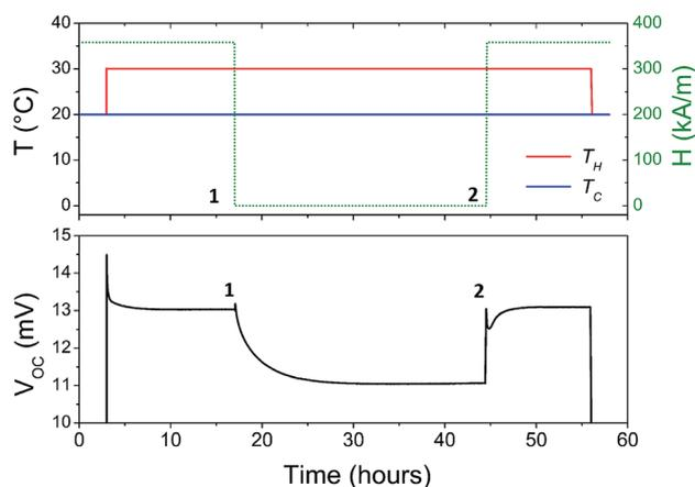
Fig. 8 Variation of apparent steady-state Seebeck voltage in the  $\phi = 0.28\%$  sample. The magnetic field is decreased from  $360 \text{ kA m}^{-1}$  to  $0 \text{ kA m}^{-1}$  (point 1) and increased again (point 2) while maintaining  $\Delta T = 10 \text{ K}$ . The results are reproducible.
