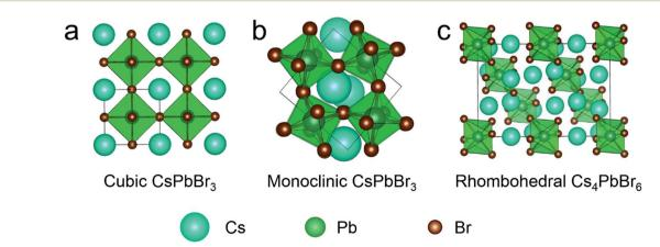
Fig. 1 Simulated crystal structure of (a) cubic CsPbBr<sub>3</sub>, (b) monoclinic CsPbBr<sub>3</sub> and (c) rhombohedral Cs<sub>4</sub>PbBr<sub>6</sub>.
