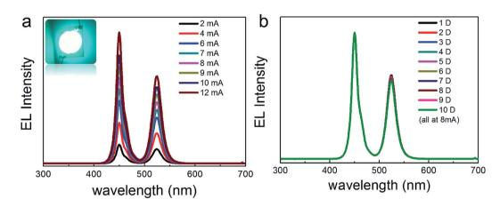
Fig. 9 (a) EL spectra of the CsPbBr<sub>3</sub>@Cs<sub>4</sub>PbBr<sub>6</sub> NC powder-based backlit LED under different currents; inset is the photograph of the backlit LED. (b) EL spectra of the CsPbBr<sub>3</sub>@Cs<sub>4</sub>PbBr<sub>6</sub>-based backlit LED lighted for 10 days under ambient conditions.
