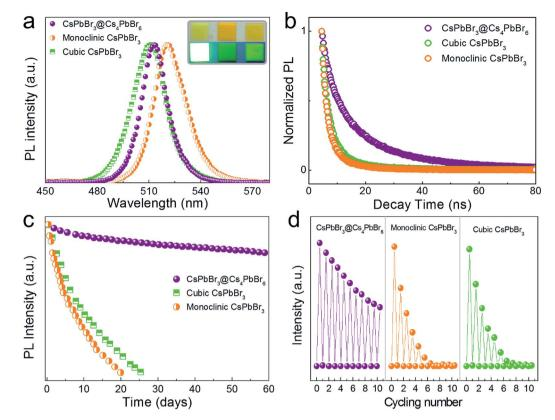
Fig. 7 (a) PL spectra and inset photographs (from left to right) of CsPbBr<sub>3</sub>@Cs<sub>4</sub>PbBr<sub>6</sub>, monoclinic CsPbBr<sub>3</sub> and cubic CsPbBr<sub>3</sub> films (mixing with PDMS). (b) PL decays of CsPbBr<sub>3</sub>@Cs<sub>4</sub>PbBr<sub>6</sub>, monoclinic CsPbBr<sub>3</sub> and cubic CsPbBr<sub>3</sub> and
