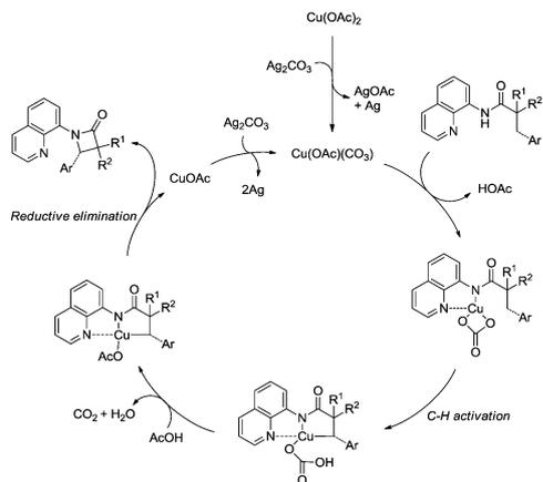
Scheme 32 The mechanism for copper(II)-catalyzed cyclization by Kanai.
