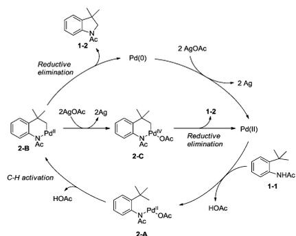
Scheme 2 The mechanism for cyclization of anilines.
