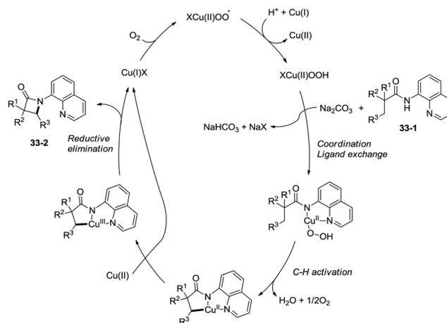
Scheme 34 The mechanism using oxygen as an oxidant.
