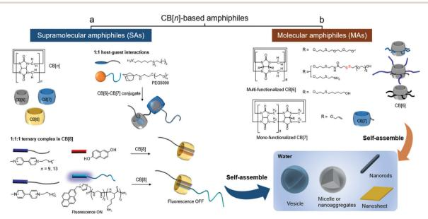
Fig. 1 Types of CB[n]-based amphiphiles: (a) supramolecular amphiphiles (SAs) formed by CB[n]-based host-guest interactions and (b) molecular amphiphiles (MAs) of CB[n] derivatives
