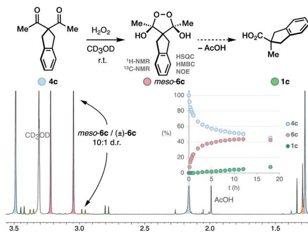
**Scheme 3** Speciation of the reaction between diketone **4c** and H<sub>2</sub>O<sub>2</sub>.
