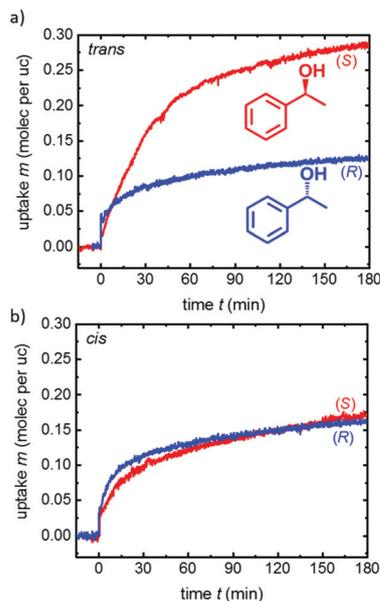
Fig. 3 Enantiopure uptakes of (R)- and (S)-phenylethanol by the  $\text{Cu}_2(\text{DCam})_2(\text{AzoBiPyB})$  film in the *trans* state (a) and *cis* state (b). The uptake is determined with a quartz crystal microbalance (QCM) in combination with a gas flow system. The molecular structures of (R)- and (S)-phenylethanol are sketched in the inset in (a).
