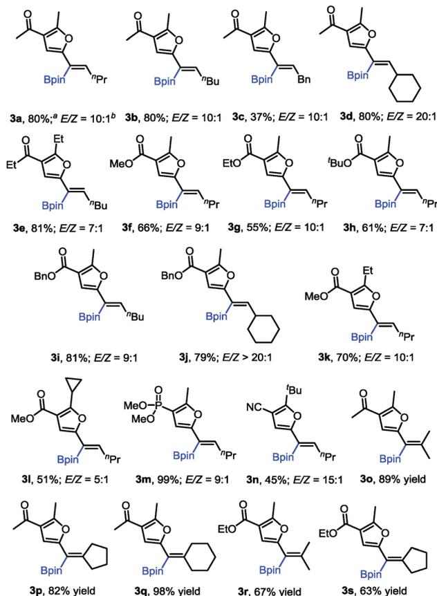
Scheme 2 Scope of the enynones. Reaction conditions: **1a–g** (0.2 mmol), **2a** (0.4 mmol), Pd(OAc)<sub>2</sub> (2 mol%), PPh<sub>3</sub> (5 mol%), <sup>i</sup>Pr<sub>2</sub>NEt (0.4 mmol), and 2,6-DMBQ (0.4 mmol) in MeOH (4 mL) at 40 °C for 10 h. <sup>a</sup> Isolated yields using column chromatography. <sup>b</sup> The *E/Z* ratio was determined by <sup>1</sup>H NMR.
