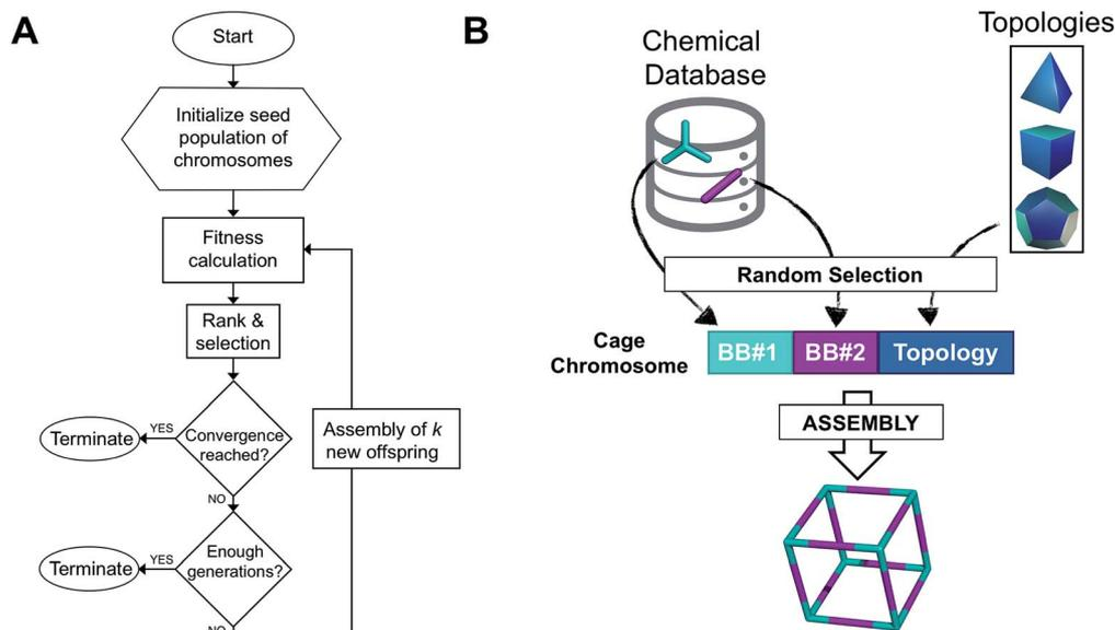
Fig. 1 (A) Overall workflow of the EA for porous organic cages. *k* represents the number of offspring individuals that temporarily extend the population size at each generation. (B) Definition of the cage chromosome, which is composed of three genes, BB#1, BB#2 and a topology. Both BBs are randomly selected from a chemical database, whereas the topology is selected from a list of feasible topologies depending on the topology of the BB. The cage is then assembled into a molecular cage structure.
