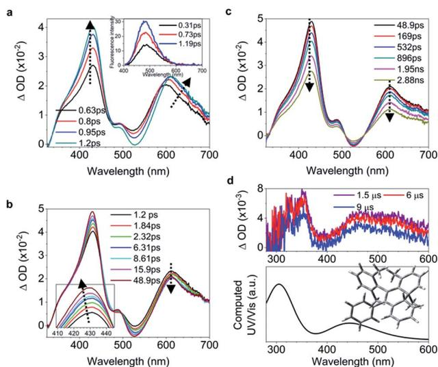
Fig. 3 Excited state dynamics of **3** in solution observed by ultrafast time-resolved spectroscopy. (a–c) Fs-TA spectra and femtosecond time-resolved fluorescence spectra (inset in (a)). (d) Ns-TA spectra (upper panel). The inset shows the calculated electronic absorption spectrum (lower panel) of the optimized structure of the photocyclized intermediate **3-IM**.
