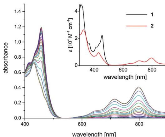
Fig. 2 Spectral evolution during photoconversion of **1** to **2** [ $c$  (**1**) =  $0.05 \text{ mM}$ ;  $c$  ( $\text{NEt}_3$ ) =  $1.4 \text{ M}$ ;  $\lambda = 457 \text{ nm}$ , DMF]. Inset: electronic spectra of **1** (black trace;  $\text{CH}_2\text{Cl}_2$ ) and **2** (red trace; THF).
