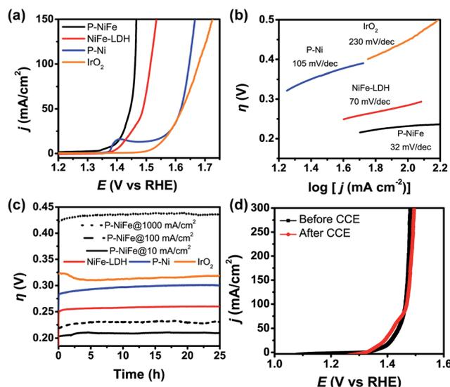
Fig. 5 (a) IR-corrected LSV curves, with a scan rate of 5 mV s<sup>-1</sup>. (b) Tafel plots for OER in 1.0 M KOH and (c) current density traces of CCE at 10 mA cm<sup>-2</sup> (as well as 100 and 1000 mA cm<sup>-2</sup> for P-NiFe, dashed line). (d) LSV curves of P-NiFe before (black square) and after (red circle) CCE for OER at 10 mA cm<sup>-2</sup> for 25 h. Catalysts: P-NiFe (black), NiFe-LDH (red), P-Ni (blue) and IrO<sub>2</sub> (orange).
