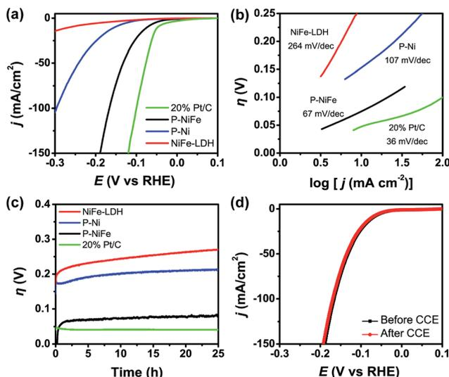
Fig. 3 (a) IR-corrected linear sweep voltammetry (LSV) curves, with a scan rate of  $5 \text{ mV s}^{-1}$ . (b) Tafel plots and (c) current density traces of CCE at  $10 \text{ mA cm}^{-2}$  for HER in 1.0 M KOH. (d) LSV curves for P-NiFe before (black line) and after (red line) CCE for HER at  $10 \text{ mA cm}^{-2}$  for 25 h. Catalysts: P-NiFe (black), NiFe-LDH (red), P-Ni (blue) and 20% Pt/C (green).
