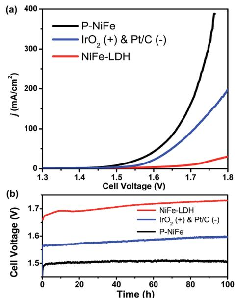
Fig. 7 (a) LSV curves of P-NiFe (black) and NiFe-LDH (red) as HER and OER bifunctional catalysts in 1.0 M KOH solution for overall water splitting. IrO<sub>2</sub> and Pt/C as OER and HER benchmarks were measured for comparison (blue). (b) Current density traces of CCE at 10 mA cm<sup>-2</sup> for overall water splitting in 1.0 M KOH for P-NiFe (black), NiFe-LDH (red), and commercial benchmarks of IrO<sub>2</sub> and 20% Pt/C (blue).
