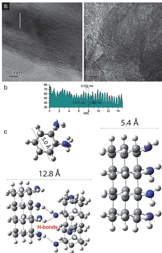
Fig. 4 (a) BF-TEM images at two different magnifications (see inset scale bars) of the recovered material presenting striations spaced at  $\sim 4$  to  $5.1$  Å and extending in the longitudinal dimension tens of nanometers. (b) A line profile measured along the white line in the low magnification BF-TEM image (a – left). (c) Views of the optimized DFT geometry structure of the one-dimensional aniline-derived nanothreads with relative dimensions.
