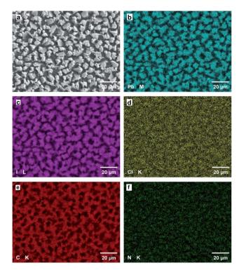
Fig. 5 (a) SEM image of the  $CH_3NH_3PDI_3(CI)$  cell without  $NH_4CI$ , and corresponding elemental mapping images of the (b) Pb M line, (c) I L line, (d) Cl K line, (e) C K line, and (f) N K line.
