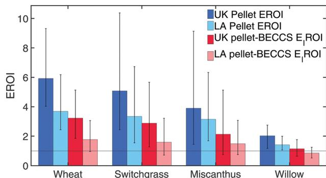
Fig. 5 Lifetime EROI of biomass pellets (blue) and lifetime  $E_1$ ROI of abated bioelectricity (red) for the two case studies. The lifetime cumulative EROI vary from 1.1 to 10.4, whereas the lifetime cumulative  $E_1$ ROI values drop to between 0.5 to 5.7.
