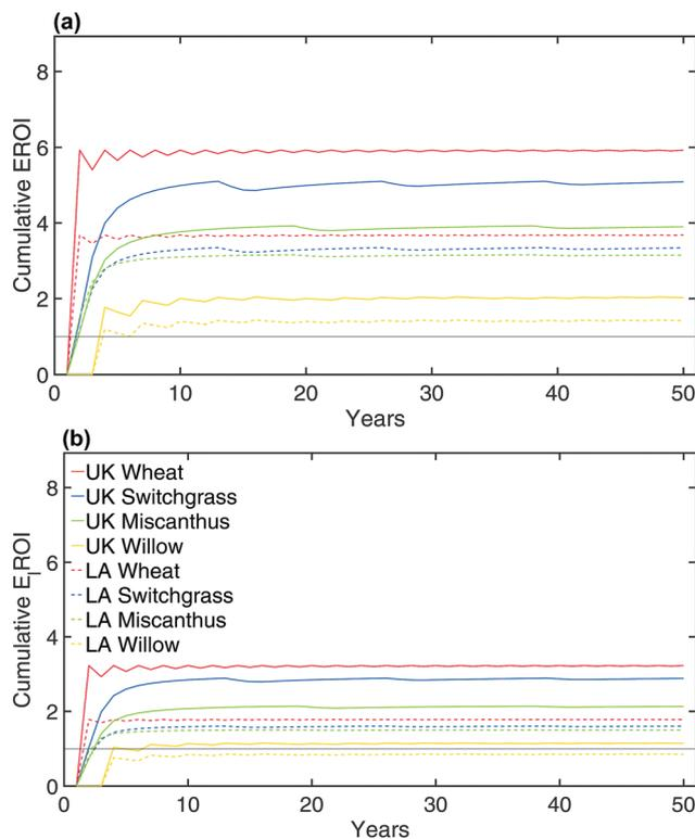
Fig. 4 Dynamic EROI of biomass pellets (top) and dynamic  $E_1$ ROI of abated bioelectricity (bottom) for the two feedstock case studies, in the median scenario. In the case of willow, upon importing pellets as opposed to using domestic pellet, the system becomes energy negative, as the lifetime  $E_1$ ROI is found below one. For energy positive systems, the  $E_1$ PBT varies from 1 to 4 years.
