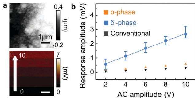
**Fig. 5** PFM characteristics of various nanowire phases. (a) Height (above) and amplitude (below) mapping of the template's top surface filled with  $\delta'$ -phase nanowires. (b) Piezoelectric response amplitude of  $\alpha$ -phase (orange),  $\delta'$ -phase (blue) and conventional (black) nanowires as a function of AC amplitude.
