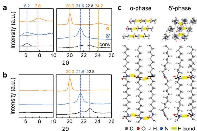
Fig. 2 XRD patterns of Nylon-11 nanowires (a) without and (b) with a nanoporous AAO template:  $\alpha$ -phase nanowires (orange);  $\delta'$ -phase nanowires (blue); and nanowires by conventional method (black). (c) 3D rendered images of  $\alpha$  and  $\delta'$ -phase crystal structures: top and side views. Black arrows indicate the direction of amide dipoles.
