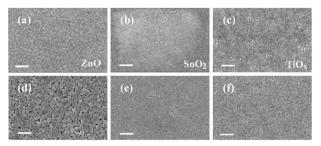
Fig. 3 SEM images of perovskite films deposited on ZnO, SnO<sub>2</sub> and TiO<sub>4</sub> substrates before (a-c) and after (d-f) vacuum-processing, respectively. The scale bar is 1 um
