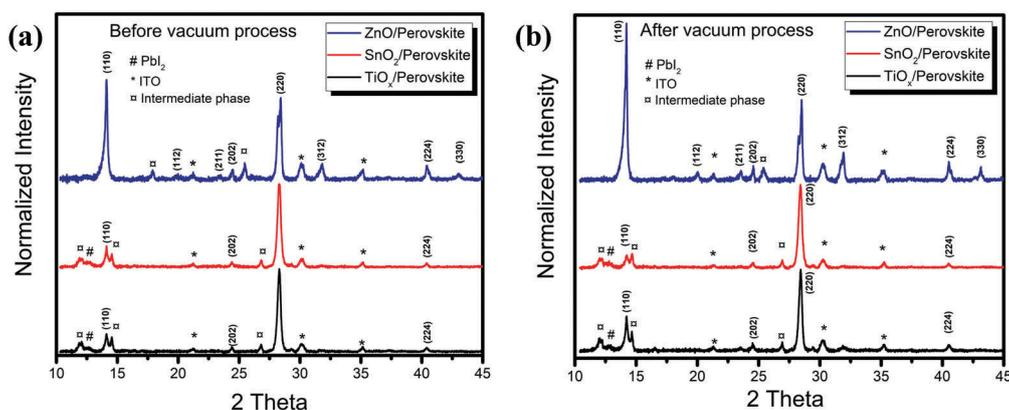
Fig. 2 X-ray diffraction patterns of perovskite films deposited on ZnO, SnO<sub>2</sub> and TiO<sub>x</sub> substrates: (a) before vacuum-processing and (b) after vacuum-processing. The XRD patterns are all normalized by the (220) peaks located at  $28.3^\circ$ .
