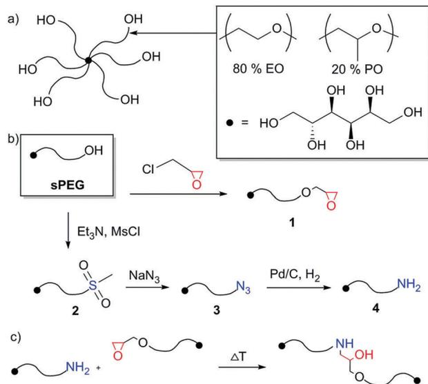
**Fig. 1** (a) The sPEG backbone contains a defined ratio of EO and PO moieties, inhibiting the crystallization at elevated molecular weight; (b) synthesis procedure for the production of sPEG-NH<sub>2</sub> and sPEG-epoxy (detailed procedures are provided in the ESI<sup>†</sup>); (c) gelation mechanism: a nucleophilic addition of amine to epoxy function.
