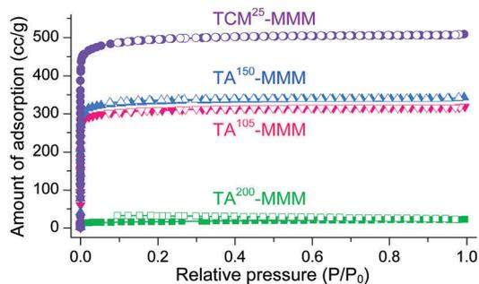
Fig. 19 N<sub>2</sub> adsorption/desorption isotherms of TA<sup>105</sup>-, TA<sup>150</sup>-, TA<sup>200</sup>-, and TCM<sup>25</sup>-MMM. The isotherms for the TCM<sup>25</sup>-MMM sample were measured after applying vacuum at room temperature for 4 h. Reprinted (adapted) with permission from ref. 70. Copyright (2018) American Chemical Society.
