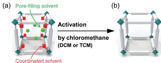
Fig. 1 Schematic illustrations of a typical unit cell of a metal–organic framework (MOF) (a) before and (b) after eliminating coordinated solvent and pore-filling solvent by chloromethane treatment.
