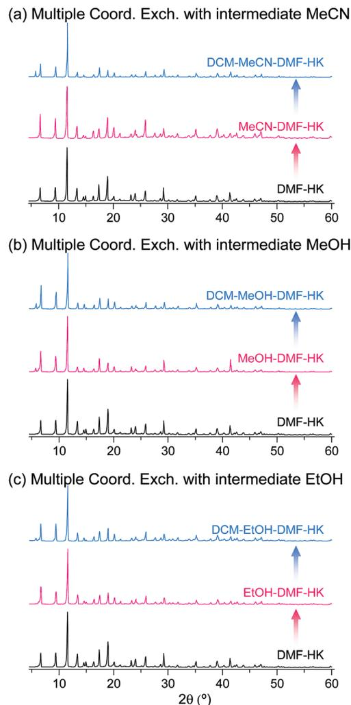
**Fig. 12** PXRD patterns of DMF-coordinated HKUST-1 before and after initial solvent treatment with (a) MeCN, (b) MeOH, and (c) EtOH and subsequent solvent treatment with DCM. Reprinted (adapted) with permission from ref. 69. Copyright (2017) American Chemical Society.
