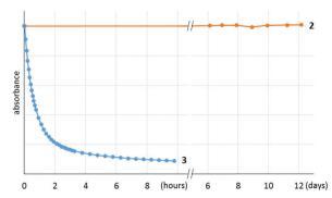
Fig. 3 Decay of the radicals 2 and 3 in wet benzene solution under air; monitored by UV-vis.
