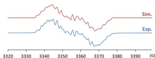
Fig. 2 Experimental (bottom) and simulated (top) EPR spectra of **2** ( $g = 2.0107$ ; hyperfine coupling constants:  $a(^{14}\text{N}) = 23.4, 9.1, 6.9 \text{ MHz}$ ,  $a(^{11}\text{B}) = 6.7 \text{ MHz}$ ,  $a(^1\text{H}) = 5.3, 3.6 \text{ MHz}$ ,  $a(^{19}\text{F}) = 2.6, 1.7 \text{ MHz}$ ).
