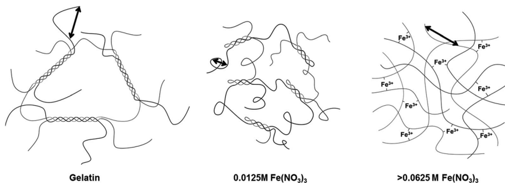
Fig. 6 Schematic showing the proposed structure of the gel at various Fe : gelatin ratios with arrows indicating the correlation length initially decreasing and then increasing as the polymer contracts and then swells.
