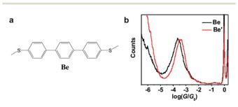
Fig. 3 (a) Molecular structure of molecule **Be** for the control experiment. (b) Conductance histograms of molecule **Be** with (red) and without (black) TFA.
