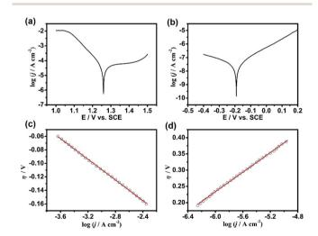
Fig. 2 (a and b) The Tafel curves of a 2 mm-diameter Pt electrode and n-GaAs electrode with area of 0.6 cm² in the working solution containing 0.040 mol L $^{-1}$  KMnO $_{\!4}$  and 1.84 M H $_{\!2}$ SO $_{\!4}$  at 35–37 °C. (c and d) The semi-logarithmic relationship between the overpotential and the current for the Pt electrode and n-GaAs electrode.
