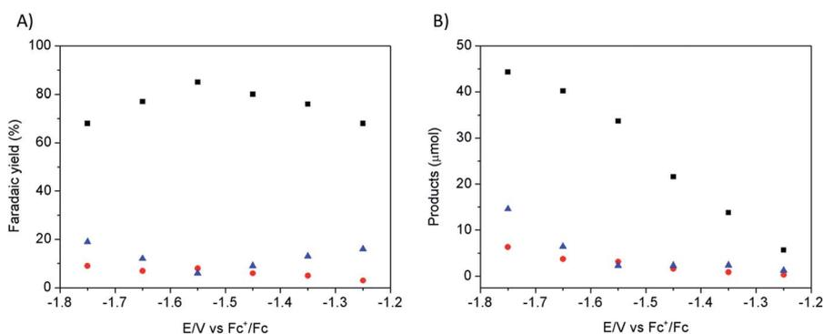
Fig. 2 CO<sub>2</sub> reduction products recorded on a modified Cu electrode (80 s electrodeposition) as a function of applied potential: faradic yields (A) and absolute amounts (B) of formate (black squares), CO (red circles) and H<sub>2</sub> (blue triangles) during 30 minutes electrolysis in CO<sub>2</sub>-saturated [EMIM](BF<sub>4</sub>)/H<sub>2</sub>O (92/8 v/v).
