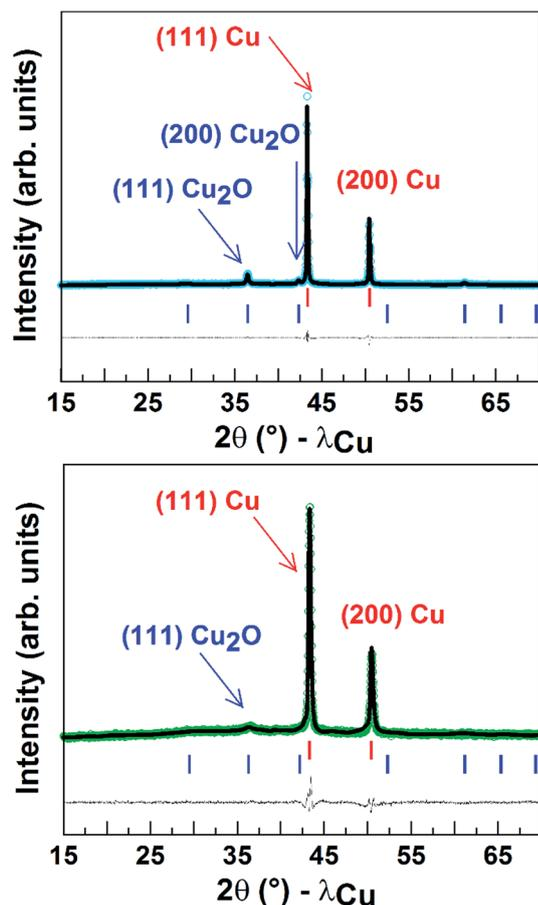
Fig. 5 Rietveld refinement of X-ray patterns of a powder of the Cu porous material (80 s electrodeposition) before (top) and after (below)  $\text{CO}_2$  electroreduction. The observed (open circles), calculated (black line) and difference (blue line on top and green line on bottom) patterns are shown. The red and blue vertical tick bars represent the Bragg positions for Cu and  $\text{Cu}_2\text{O}$ , respectively.
