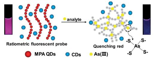
Scheme 2 Schematic illustration of the ratiometric fluorescent sensors for the detection of As( $\parallel$ ), the insets show the corresponding fluorescent photo under 365 nm UV lamp from fushia (left) to blue (right) upon the addition of As<sup>3+</sup> in the sensing system.
