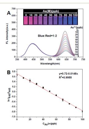
Fig. 2 (A) The fluorescent spectra of mixture of blue CDs and red QD chains at ratios 1:2 with the addition of As(III). The insets show the corresponding fluorescent photo under 365 nm UV lamp. (B) Fluorescent intensity ratio, In ( $I_{640}/I_{445}$ ), vs. the concentrations of As(III) in the TTCA-QD chains/CDs.
