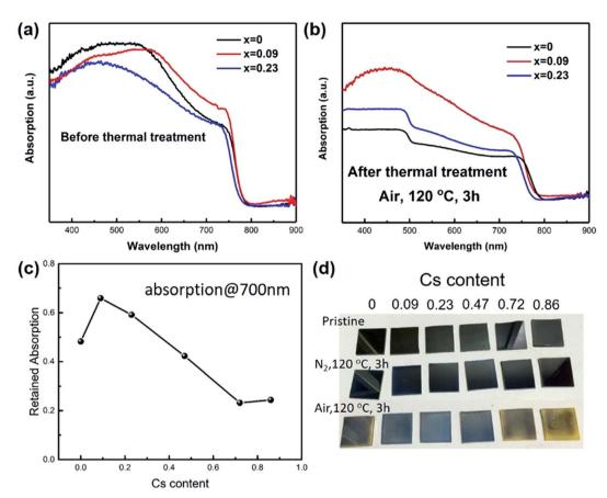
Fig. 1 Thermal stability study of perovskite films with different Cs content. (a) Perovskite films with compositions of  $Cs_x MA_{1-x}Pbl_3$  before thermal treatment, where x represents Cs content. (b) Perovskite films after thermal treatment at 120 °C for 3 hours exposing to air. (c) Retained absorption at 700 nm for perovskite films with x ranging from 0 to 0.86. (d) Photographs of perovskite films exposing to different atmosphere.
