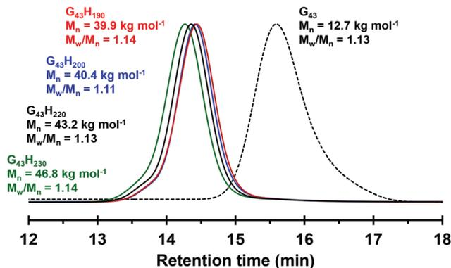
Fig. 1 DMF chromatograms obtained for MPETTC-PGMA<sub>43</sub> macro-CTA (black dotted curve) and the corresponding MPETTC-PGMA<sub>43</sub>-PHPMA<sub>y</sub> diblock copolymer vesicles ( $y = 190, 200, 220$  and  $230$ ). Molecular weight data are calculated relative to a series of near-monodisperse poly(methyl methacrylate) calibration standards. G and H denote poly(glycerol monomethacrylate) and poly(2-hydroxypropyl methacrylate), respectively.
