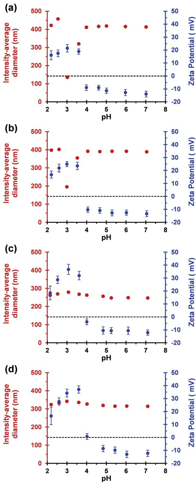
Fig. 4 Intensity-average diameter vs. pH and zeta potential vs. pH curves obtained for MPETTC-PGMA<sub>43</sub>-PPHMA<sub>y</sub> diblock copolymer nano-objects where  $y =$  (a) 190, (b) 200, (c) 220 and (d) 230. All measurements were made at 20 °C for 0.1% w/w copolymer dispersions prepared in the presence of 1 mM KCl background salt.
