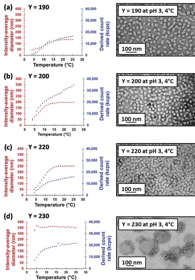
Fig. 6 Variation in intensity-average diameter and derived count rate vs. temperature on cooling a 0.1% w/w aqueous dispersion of MPETTC-PGMA<sub>43</sub>-PHPMA<sub>y</sub> diblock copolymer nano-objects at pH 3 from 20 °C to 4 °C and the corresponding TEM images obtained on drying at 4 °C for y values of (a) 190, (b) 200, (c) 220 and (d) 230.
