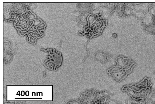
Fig. 3 Representative TEM image obtained for the transient 'jellyfish' intermediate structures formed by an MPETTC-PGMA<sub>43</sub>-PHPMA<sub>190</sub> diblock copolymer after 24 h at pH 3.0.
