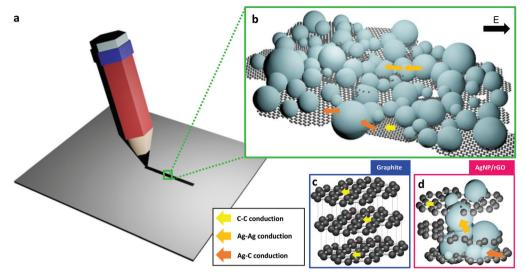
Fig. 2 (a) Schematic images of a pencil-drawn line. (b) Schematic illustration describing a detailed conduction mechanism of the AgNPs/rGOdrawn trace. Three different colored arrows are to explain three different paths for electron transport. Electrical conduction of (c) graphite and (d) AgNPs/rGO could be compared.
