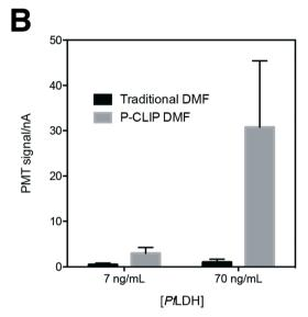
Fig. 5 DMF immunoassay for PfLDH. (A) Standard curve for PfLDH as determined by traditional DMF-ELISA. Error bars represent  $\pm$  1 std. dev. (n=3). (B) Comparison of mean signals obtained by traditional DMF-ELISA (black) and P-CLIP modified DMF-ELISA (grey) for concentrations below the limit of detection (7 ng mL $^{-1}$ ) and limit of quantitation (70 ng mL $^{-1}$ ) of the traditional DMF-ELISA. Error bars  $\pm$  1 std. dev. (n=3).
