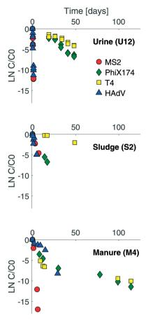
Fig. 1 Inactivation curves for MS2 (red circles), ΦΧ174 (green diamonds), T4 (yellow squares) and HAdV (blue triangles) in stored urine (U12), sludge (S2) and manure (M4). The complete set of inactivation curves obtained in this study are shown in the ESI† (Fig. S2 and S3).
