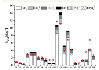
Fig. 3 Contribution of the main bases present in stored urine, sludge and manure to the  $k_{\rm pred}$  of MS2. The measured  $k_{\rm obs}$  is depicted by the
