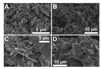
SEM images of hydrothermally synthesized PBIs and PBA. (A) Hydrothermally treated PBA (24 h, 200 °C). (B-D) n-C $_n$ -PBIs obtained hydrothermally (24 h, 200 °C). B = n-C<sub>5</sub>-PBI, C = n-C<sub>8</sub>-PBI, D = n-C<sub>12</sub>-PBI
