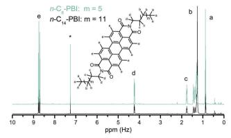
Fig. 3  $^{1}$ H-NMR spectra (600 MHz, CDCl<sub>3</sub>/TFA: 5/1 v/v, 16 scans) of n-C $_n$ -PBIs synthesized hydrothermally at 200  $^{\circ}$ C for 24 h; black = n-C $_{14}$ -PBI, turquoise = n-C $_{8}$ -PBI. Solvent residual peak (7.26 ppm) is marked with \*.
