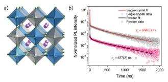
Fig. 9 (a) Crystal structure of Cs<sub>2</sub>BiAgBr<sub>6</sub>. Adapted with permission from ref. 427. Copyright 2015, American Chemical Society. (b) Time-resolved room temperature photoluminescence (PL) of single-crystal and powder Cs<sub>2</sub>BiAgBr<sub>6</sub>, including fits for the PL decay time (τ). Reprinted with permission from ref. 428. Copyright 2016, American Chemical Society
