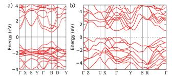
Fig. 5 Band structures of germanium-based solar absorbers: (a) CH<sub>3</sub>NH<sub>3</sub>Gel<sub>3</sub>—adapted with permission from ref. 240. Copyright 2015, American Chemical Society—and (b) GeS. Adapted with permission from ref. 241, Copyright 2013, American Physical Society.
