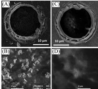
Fig. 2 Scanning electron micrograph (SEM) images for (A, B) a cellulose film deposit and (C, D) a chitosan-doped cellulose film deposit on a 20  $\mu$ m diameter microhole in a PET film.
