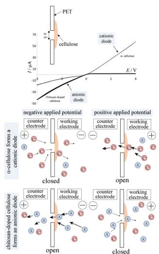
Cyclic voltammetry (scan rate: 20 mV s<sup>-1</sup>) of  $\alpha$ -cellulose only films (dotted line) and chitosan-doped cellulose films (black solid line) on a 20 µm diameter microhole in a PET sheet in 50 mM NaCl on both sides of the membrane. The schematic drawing shows the four mechanistic cases of a cationic diode and an anionic diode under positive potential and negative potential polarisation, respectively.
