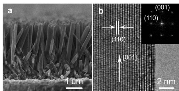
Fig. 1 Morphologies of rutile TiO<sub>2</sub> NW arrays. (a) Cross-sectional field emission scanning electron microscopy (FE-SEM) image of NW arrays with an average diameter and length of about 100 nm and 3 μm, respectively. (b) High-resolution transmission electron microscopy (HR-TEM) image of a typical NW. The NW has a growth direction of [001] and side surfaces of {110} crystal plane. The inset in panel (b) is the selected area electron diffraction pattern of the NW.
