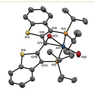
Fig. 4 Molecular structure of  $1 \cdot OH$ . Hydrogen atoms have been omitted for clarity. Displacement ellipsoids are shown at the 50% probability level. Selected bond lengths (Å): Ir(1)-P(1), 2.3110(10); Ir(1)-P(2), 2.3135(10); Ir(1)-C(1), 2.078(4); Ir(1)-O(1), 2.084(3); Ir(1)-O(2), 1.972(4); C(1)-O(1), 1.359(5). Selected bond angles (°): C(1)-Ir(1)-O(1), 38.12(13); C(1)-O(1)-Ir(1), 70.7(2); Ir(1)-C(1)-O(1), 71.2(2); P(1)-Ir(1)-P(2), 166.23(4).
