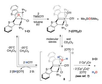
Scheme 7 Model reactions for water elimination.
