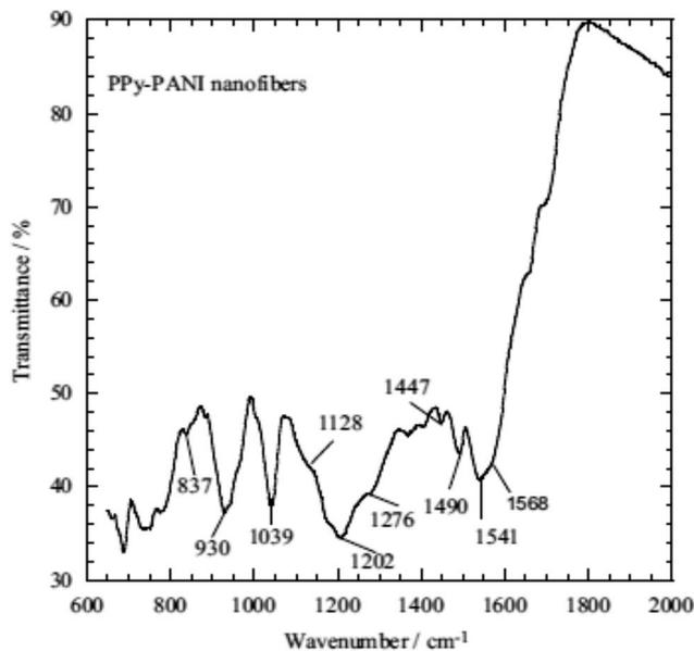
Fig. 5 The ATR-FTIR spectrum of the PPY-PANI nanofibers.<sup>33</sup>
