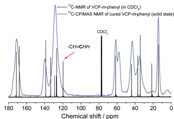
**Fig. 5**  $^{13}\text{C}$ -NMR comparison:  $^{13}\text{C}$  NMR ( $\text{CDCl}_3$ , 75 MHz) of un-cured VCP-*m*-phenyl and  $^{13}\text{C}$ -CP/MAS NMR (100 MHz) of cured VCP-*m*-phenyl. The signal at 119.7 ppm defines the carbon atom of the terminal vinyl bond. After curing within the  $^{13}\text{C}$ -CP/MAS NMR spectra only a shoulder, hardly perceived at 119.7 ppm, is observed, which indicates a high cross-linking density of the cured VCP-*m*-phenyl.
