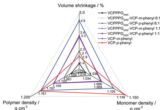
**Fig. 6** Spider chart showing the dependency between the monomer- and polymer density to the volume shrinkage. Only the partial-crystalline VCP-*p*-phenyl shows a disproportion within the correlation, based due to the denser partial-crystalline monomer structure of VCP-*p*-phenyl ( $1.139\text{ g cm}^{-3}$ ).
