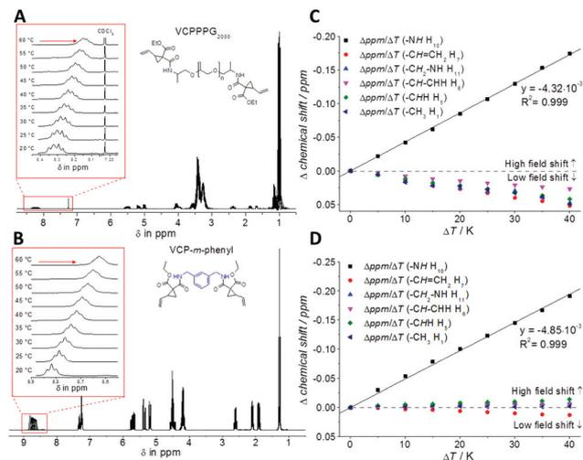
**Fig. 2** (A + B) Variable-temperature <sup>1</sup>H-NMR experiments of VCP-PPG<sub>2000</sub> and VCP-*m*-phenyl (0.5 mM in CDCl<sub>3</sub>) between 20–60 °C. (C + D) Graphical plot of chemical shift within <sup>1</sup>H-NMR experiments. With increased temperature a decreased deshielding effect is anticipated, as a partial rupture of the H-bonds occurs.
