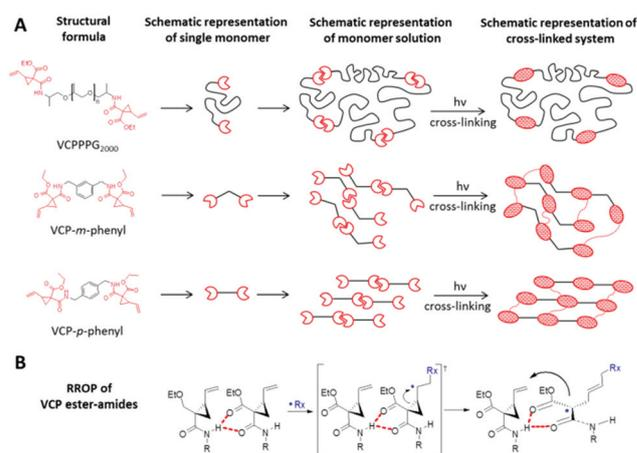
**Fig. 1** (A) Schematic aspect of the H-bond mediated partial self-assembly of VCP ester–amide units. The alignment is primary taking place at the functional group. (B) Proposed RROP mechanism of amide-based VCPs. The partial self-assembly and the enhanced orbital arrangements have to be taken into consideration.
