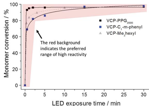
**Fig. 3** Determined monomer conversion for the photo-polymerization of VCP-PPG<sub>2000</sub>, VCP-*m*-phenyl and VCPMe<sub>3</sub>hexyl (1 mol% initiator CQ: EDMAB in a molar ratio of 1:2). The curing was performed under a controlled atmosphere of nitrogen using a commercial LED source (2.013 mW cm<sup>-2</sup> for 465 nm).
