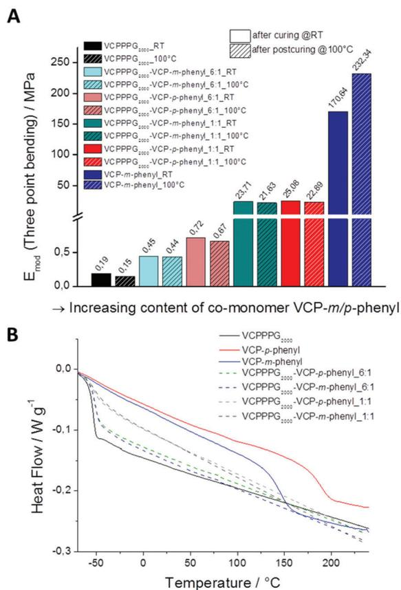
**Fig. 4** (A) Determined E-moduli of cured VCP-*m*-phenyl specimens, as well as by co-networks in ratios of 6 : 1 and 1 : 1 of VCP-*p*-phenyl. VCP-*m*-phenyl and VCP-*p*-phenyl. With increasing content of the co-monomer VCP-*m/p*-phenyl, the moduli could be raised up to 1200 times to higher values. (B) Second DSC heating trace of cured VCP specimens, illustrating the glass transition  $T_g$  of the cured samples.
