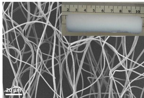
**Fig. 1** SEM image of an electrospun nanofibre mat and the digital photo of sponge made after cutting and drying (inset).
