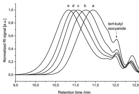
**Fig. 1** SEC chromatogram showing the growth of polyester **P1** due to addition of 5 equivalents of monomer **3** after specific time periods measured from reaction mixture; (a = first (0 h), b = second (2 h), c = third (4.5 h), d = fourth addition (7.5 h), e = 24 h).
