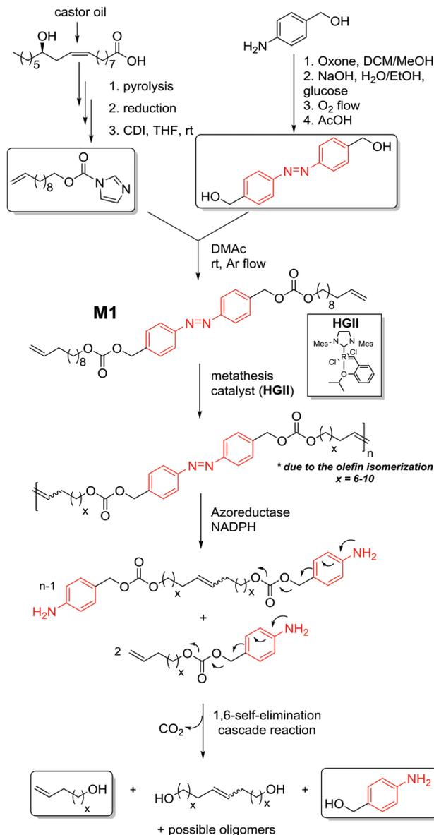
**Fig. 2** Synthesis of the monomer, **M1**, possessing a self-immolative character and the respective ADMET polymer **P1**. The plausible cleavage of azobenzene linkages in **P1** upon enzymatic action and subsequent 1,6-self elimination to smaller molecular weight species.
