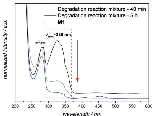
**Fig. 4** UV-visible spectra illustrating the degradation of **M1** in the presence of 5.5 equivalents of  $\text{Na}_2\text{S}_2\text{O}_4$  in a mixture of dichloromethane : methanol : water at reflux temperature (for details see section A.8 in the ESI†). Spectra recorded in THF at 25 °C.
