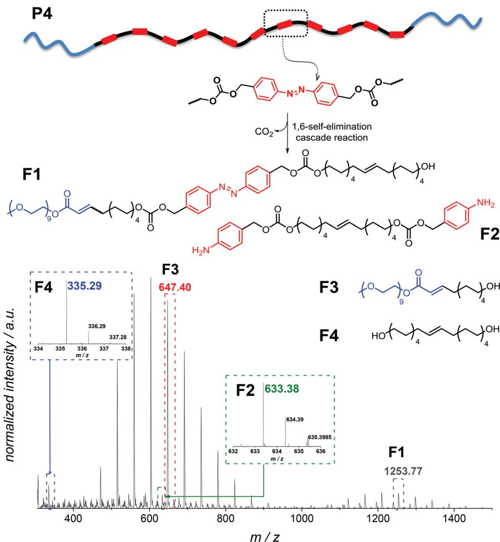
Fig. 7 High resolution ESI-MS analysis of the degradation fragments of P4 after enzymatic treatment for 24 h (P4<sup>+</sup>).
