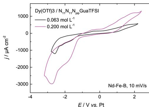
Fig. 6 CV of  $0.063$  mol  $\text{L}^{-1}$  and  $0.200$  mol  $\text{L}^{-1}$  of  $\text{Dy}(\text{OTf})_3 + \text{N}_{11}\text{N}_{11}\text{N}_{\text{pip}}\text{GuaTFSI}$  on Nd-Fe-B, recorded with a scan rate of  $10$  mV  $\text{s}^{-1}$ .
