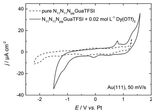
Fig. 2 CV of N $_{11}$ N $_{11}$ N $_{pip}$ GuaTFSI (dashed line) and N $_{11}$ N $_{11}$ N $_{pip}$ GuaTFSI +  $0.02 \text{ mol L}^{-1}$  Dy(OTf) $_3$  (solid line) on Au(111) at a scan rate of  $50 \text{ mV s}^{-1}$ .
