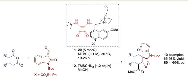
Scheme 21 Organocatalytic asymmetric Tamura cycloaddition involving a squaramide catalyst
