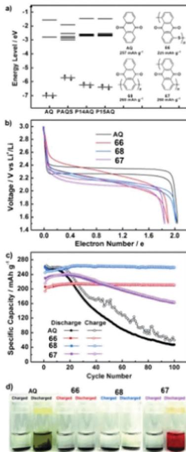
**Fig. 11** (a) Electronic configuration of anthraquinone, **66**–**68**, calculated by DFT. (b) Charging/discharging and (c) cycling performance of the electrodes fabricated using anthraquinone and compounds **66**–**68**. (d) Solubility of the charged and discharged electrodes in a 1 M LiTFSI DOL:DME 2:1 electrolyte. (Reproduced from ref. 23, reprinted with permission, copyright 2015, Wiley-VCH).
