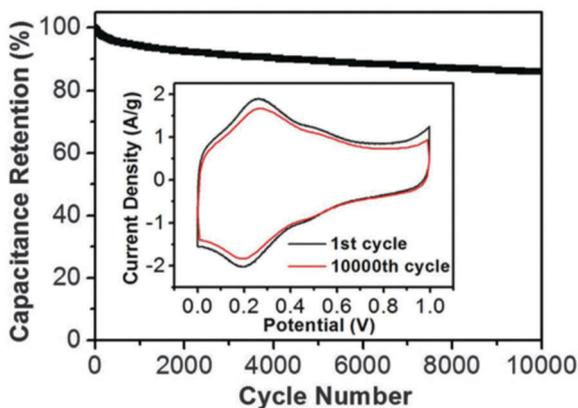
Fig. 24 Cycling stability of FGH-based SC at a current density of  $10 \text{ A g}^{-1}$ . Inset shows a cyclic voltammogram of the device at  $5 \text{ mV s}^{-1}$  after the 1st and 10 000th galvanostatic charge/discharge cycle. (Reproduced from ref. 159, reprinted with permission, copyright 2013, Wiley-VCH).
