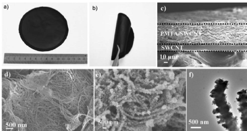
Fig. 9 (a and b) Photograph of hybrid **49**/SWCNT film, scanning electron microscope image of (c) a cross-section of the hybrid film with a SWCNT current collector, (d) the top of the bare SWCNT film, and (e) the hybrid **49**/SWCNT film. (f) Transmission electron microscope image of hybrid **49**/SWCNT film. (Reproduced from ref. 61, reprinted with permission, copyright 2015, Wiley-VCH).
