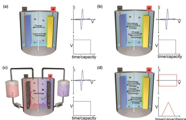
**Fig. 1** Schematic depicting the working principle of (a) metal-ion batteries, (b) dual-ion batteries, (c) redox flow batteries, and (d) supercapacitors. The insets show the ideal electrochemical behaviour of each type of device when measured using cyclic voltammetry and galvanostatic charging/discharging. Here,  $V$  is voltage and  $i$  is current.
