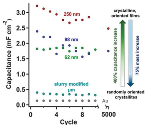
Fig. 27 Capacitance retention over 5000 cycles for **180** slurry, blank Au electrode, and oriented thin films as a function of thickness: 250 nm (red), 98 nm (blue), 62 nm (green). (Reproduced from ref. 172, reprinted with permission, copyright 2015, American Chemical Society).
